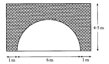
The wall is in the shape of a rectangle with a semi-circular space for the tunnel.
